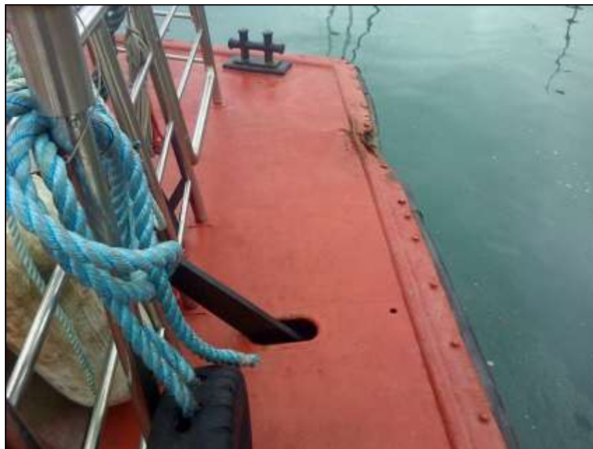
Figure 2: Contact damage to forward deck
